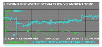
PRE-PROJECT (1<sup>ST</sup> WEEK IN FEB, 2014) Heating load due to minimum HHW valve positions for freeze protection in six HVAC units.
