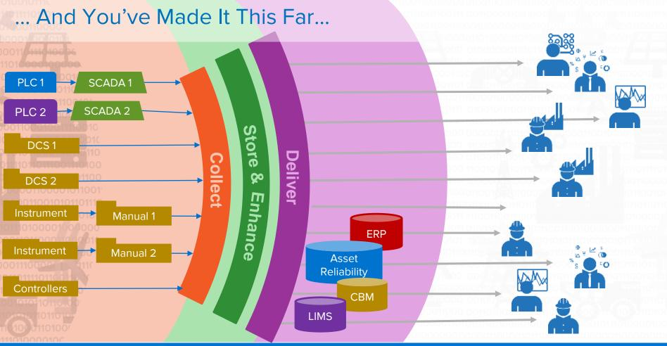
The PI System handles operational data from sensor to destination
