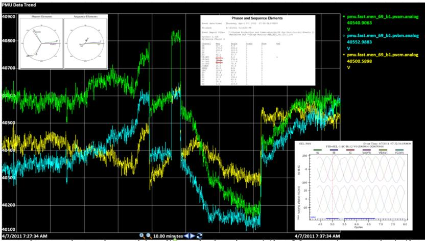
We have been observing odd voltage behavior at the Menominee substation due to a foundry load located nearby. We are using SEL triggers to identify when unbalances occur and then using PMU data to help analyze the events.
