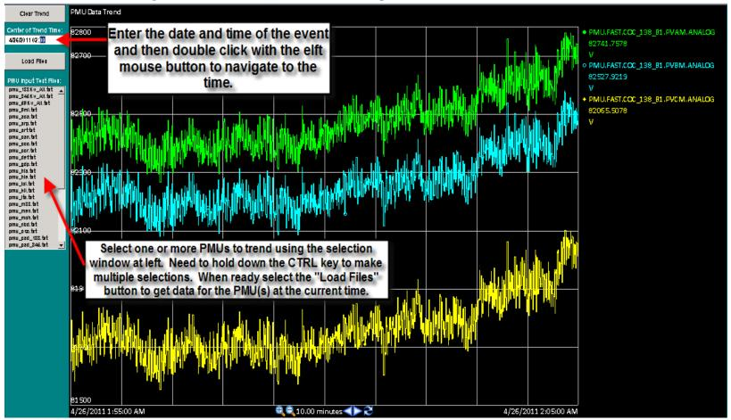
PI ProcessBook display could be used to display phase voltage data for one or more PMUs.
