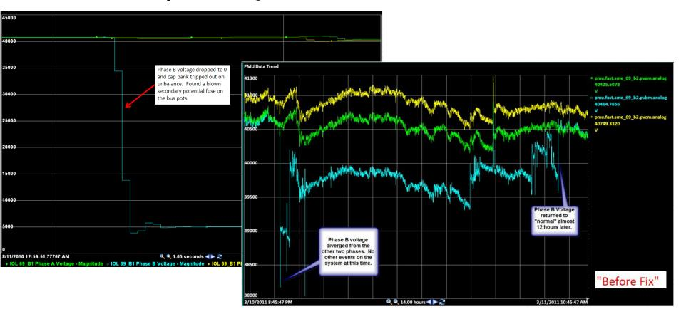
Anomalies in voltage trace data can be used to determine when there are issues with the voltage inputs used for relaying. If caught early we may be able to prevent relay misoperations due to PT fuse failures.
