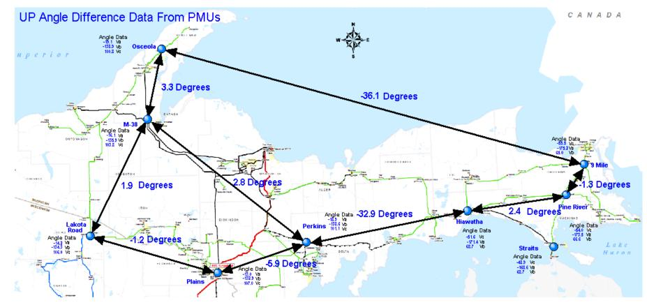
PI ProcessBook display could be used to monitor the difference in phase angles across a pre-defined system. In this example the UP is split and the phase angle across the split is around 35 degrees.
