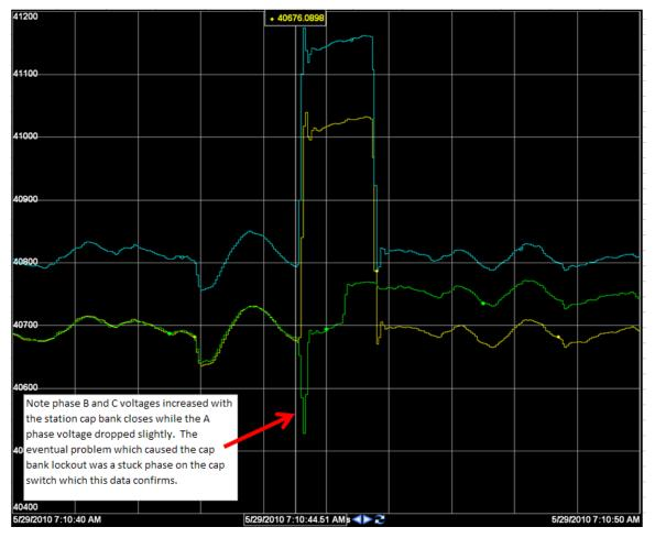
Voltage traces from a nearby station could have been used to identify a stuck phase on a cap bank switch that was closed in and eventually tripped back out.
