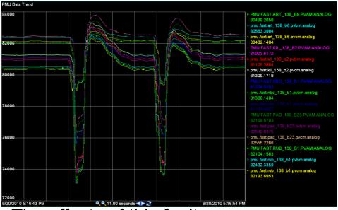
The effects of this fault were seen on the 138 Kv and 345 Kv traces from PMUs across our footprint.
