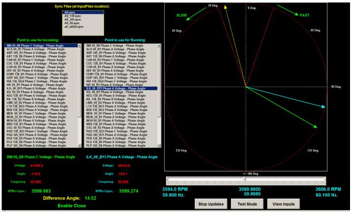
PI ProcessBook display can be used to monitor the difference in phase angles between two sites. The chart at right is trending data from the 9 Mile sub in the eastern UP [cyan trace] against the Indian Lake substation in the central UP [green trace]. The yellow dashed trace is the angle difference between the two. This could potentially be used for reconnecting electrical
