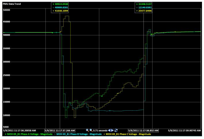
Voltage traces from a PMU located close to a line trip helped identify a slow breaker trip that was eventually traced back to a dirty breaker contact. We would not have seen this misoperation without the PMU data.
