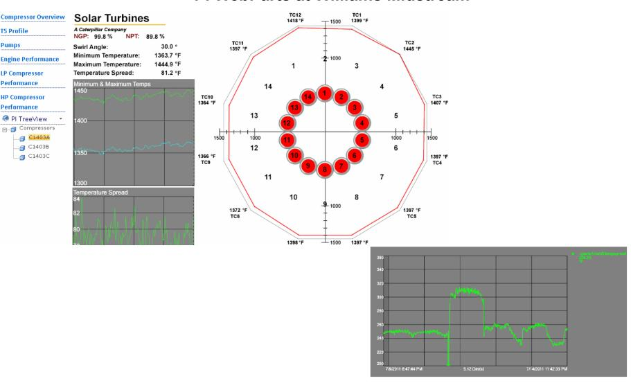
"Exhaust Temperature Profile" solution provided an immediate success story by displaying an anomaly with exhaust gas temperatures.
