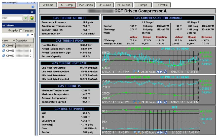
With PI ProcessBook's Element Relative feature, a single display provides visualizations for many assets.
