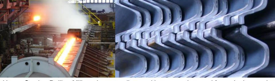
Heavy-Section Rolling Mill produces medium and heavy section steel from single round bars, through shaped profiles, up to profiles of special cross sections.
