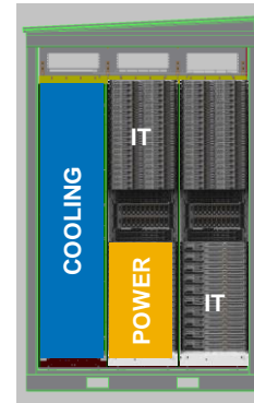
Medium density Includes power elements & UPS back-up
