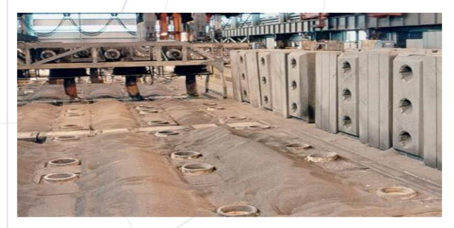
Anode baking: batch process; 14 to 17 days at a maximum temperature of 1200 C
