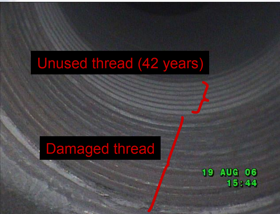
Balance plane plug thread failure
