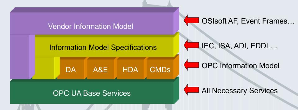
OPC UA Clients can discover Nodes in the UA Address Space and access all data from the derived layers
