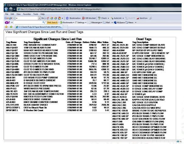
A controller that is maxed out or completely shut off will show up on the dead tags list
