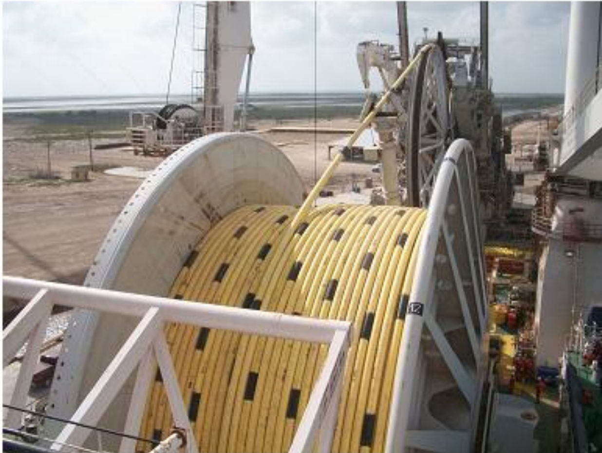
The pipe landing on the reel as seen from the bridge. The average rate for spooling is 22m of pipe per minute.
