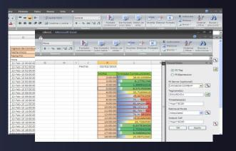
PI DataLink establishes a direct connection between the OSIsoft PI System and Microsoft Excel, with this tool we design and built reports for fuel stocks and thermal generation performance to be published in SharePoint.
