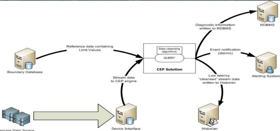
Analyze high speed process data and associated diagnostic information to identify suspect data; call routines to "cleanse" suspect data and output the processed data and diagnostic information; recognize critical events that need to be passed on immediately.
