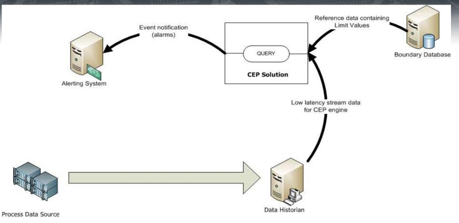
Detect pattern-based process data events (e.g. limit exceedance) in moving time windows and report the non-conformance immediately
