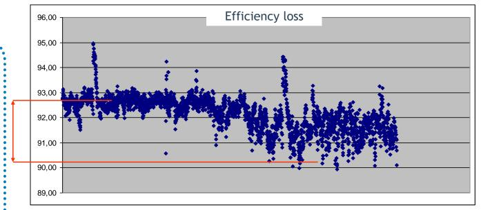
Instead of complex measurement procedure twice a year we provide online calculation (in connection with neural networks) to see how device (boiler behaves)
