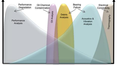
Spectrum of Failure Modes for Given Equipment
