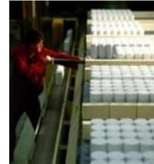
Ceramic substrates for automotive catalytic converters
