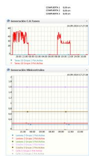
Hydraulic control and production in hydro plant.
