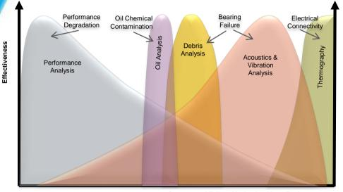
Spectrum of Failure Modes for Given Equipment
