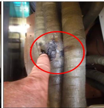
Photo 8 – Burned and Carbonized Lead Insulation
