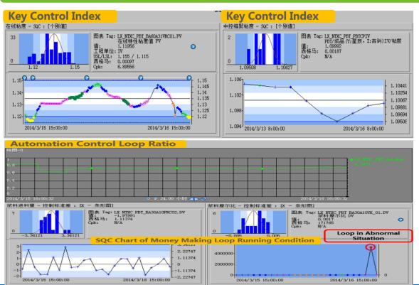
**Ensuring equipment to operate at its full potential**, using PI SQC chart to monitor the operations situation
