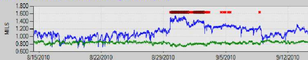
FS1:97X178I.PV, 1804 LP Shaft #2 bearing radial Vert, (MILS)
