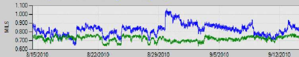
FS1:97X176I.PV, 1804 LP Shaft #2 bearing radial Horz, (MILS)
