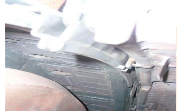
Unseated Transition Piece Floating Seal
