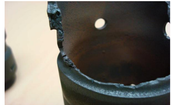
Unseated Transition Piece Floating Seal
