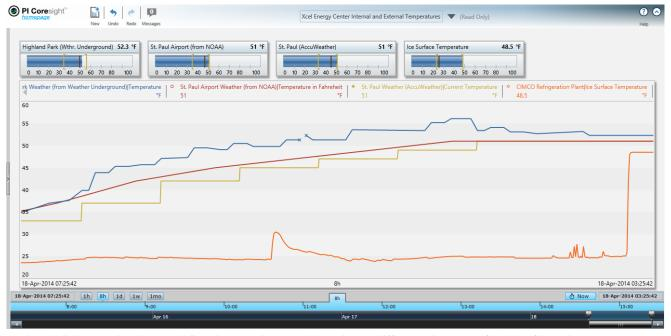
In addition to the internal Davis weather station, three different internet feeds of local external weather are also being monitored
