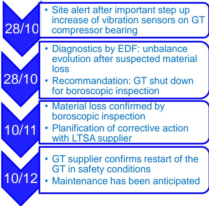
Step up increase of both vibration sensors of the bearing
