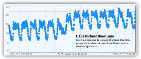
With Profile Alarms, this event would have been identified almost as soon as it started, a full day and a half before the standard threshold alarm identified it
