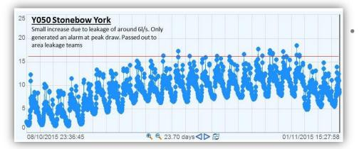
This shows a gradually increasing leak that took the threshold alarm over 6 days to detect. A profile alarm would have detected this within the first day
