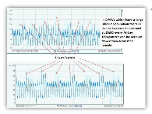
Using the feature of Profile Alarms that compensates for variations occurring at a particular time on the same day every week, these events would be filtered out. A genuine leak occurring at the same time would still be detected however, since the alarm is not inhibited, just the thresholds adjusted temporarily
