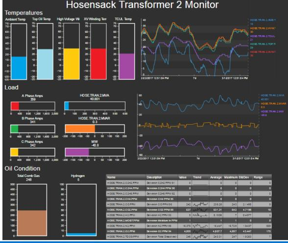
Asset Framework allows for quick and easy building of rich element relative diagnostic dashboards displaying asset condition.
