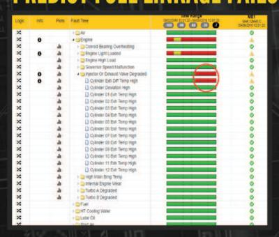
Analytics identifies a cylinder with temperatures increasing at a much greater rate than other cylinders.
