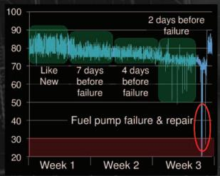
Potential problem not addressed by onboard crew - failure still occurred, resulting in repair costs and downtime.
