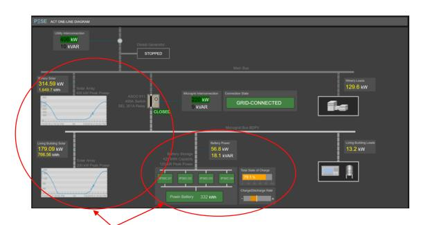
Controlled by PXiSE 8 Solar Inverters, 4 Energy Storage Inverters and 1 ASCO Switch
