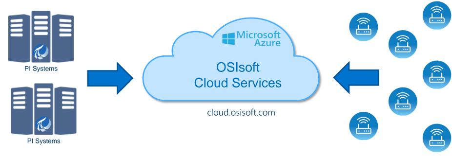
Operational data is transferred between PI Systems and OCS ... and also between Edge components and OCS.
