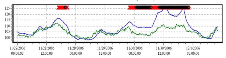
After detection, the filters were found dirty, replaced, and the real time oil level and temps dropped back to the model expected value.
