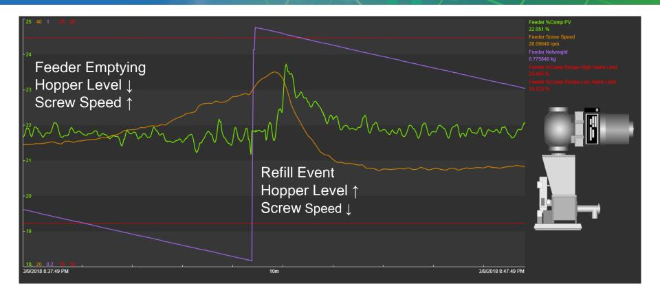
\*Screw speed ramp rate and lag critical to maintaining consistent mass flow during refills\*
