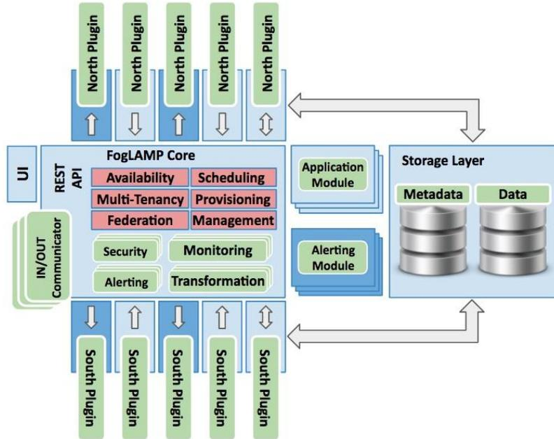
North Plugins to forward data upstream. Built in Plugins for PI Server and OSIsoft Cloud Services using PI Relay. Upstream system may also be another FogLAMP node.
