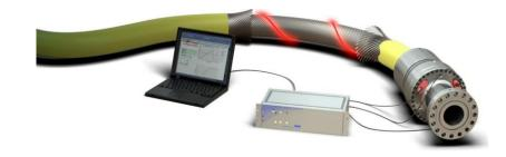
Detect the most common failure modes observed in flexible pipes!
