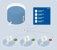
Automatic adjustment of disposal and producing wells to maintain optimal tank level
