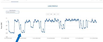
Too much net metering on weekends – solution is to potentially adjust demand profile, consider energy storage or downsize fuel cell
