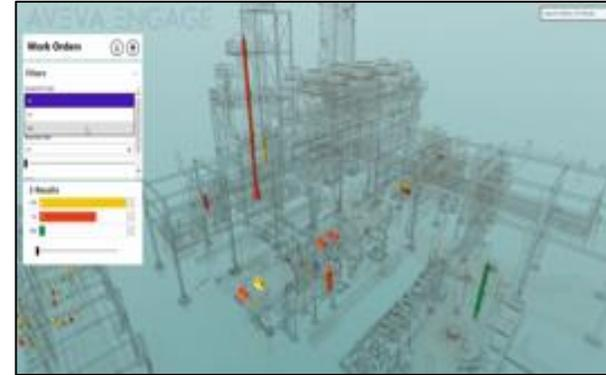
Viewing critical and supercritical equipment in the workorders highlighted on the 3D facility model.
