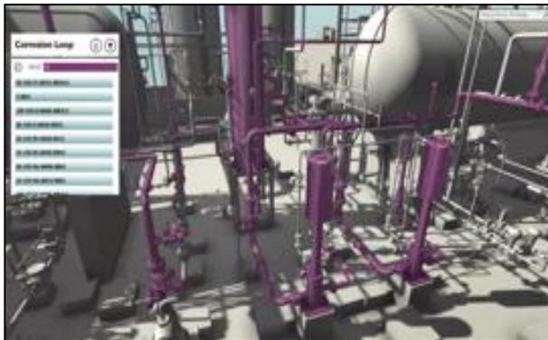
Viewing corrosion loops in the 3D model to support in inspection activity reducing the need for onsite survey.
