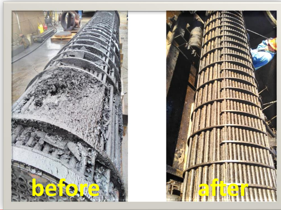
Heat Exchangers Fouling in the Field
