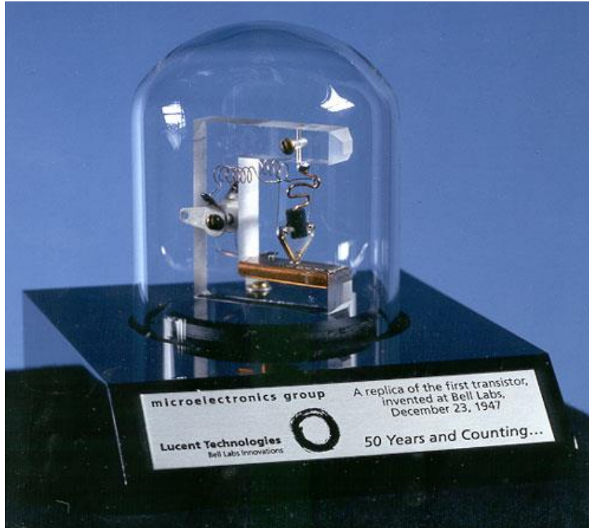
Germanium-based point-contact transistor. 1947 John Bardeen, Walter Houser Brattain, William Shockley. BELL LABS
