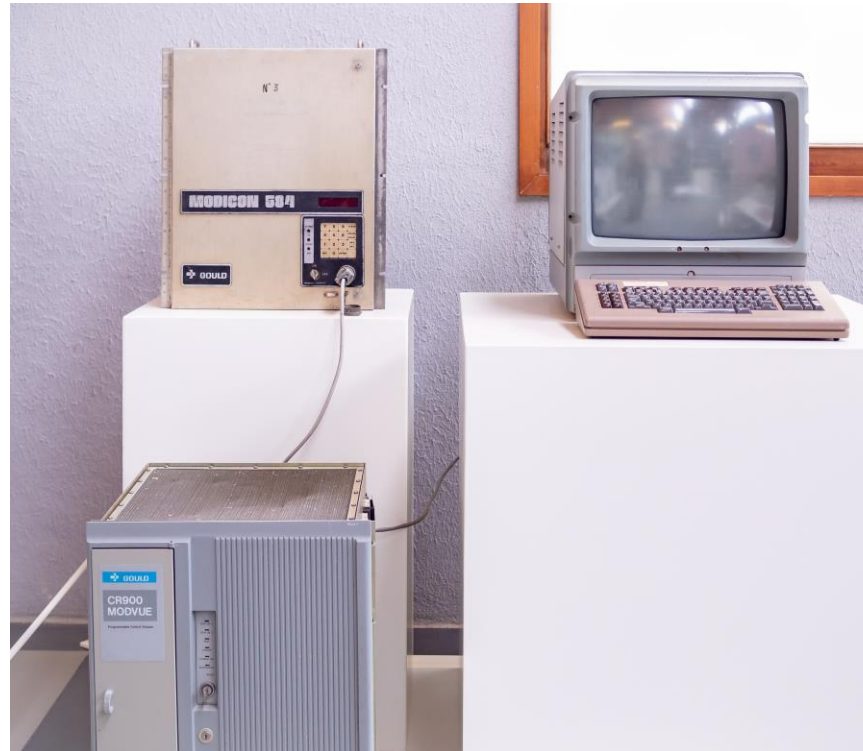
Modicon 084, the first 'Programmable Controller'. 1969 Richard Morley
