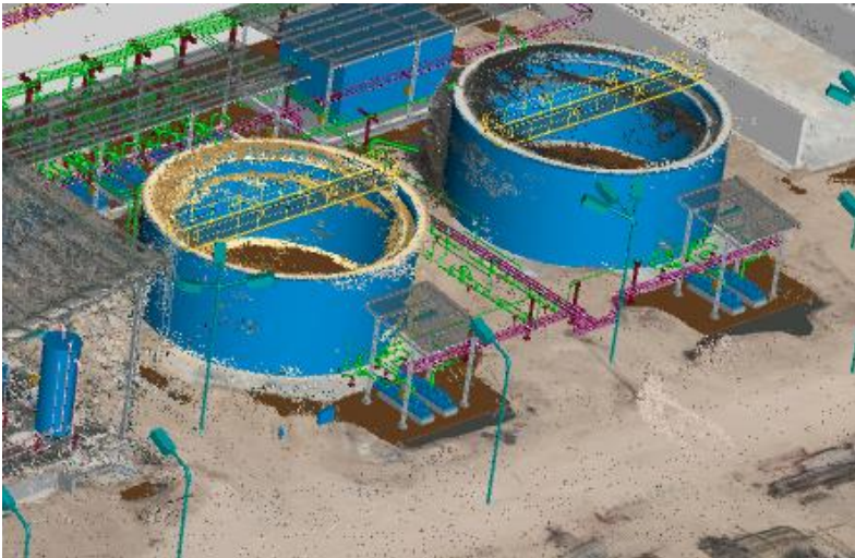
Showing Quality Check between the 3D Model and Drone Point Cloud
