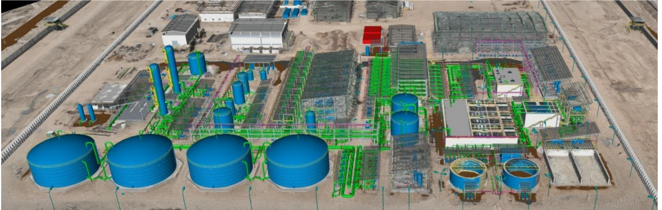
Merging 3D Model + Actual Site Drone survey
