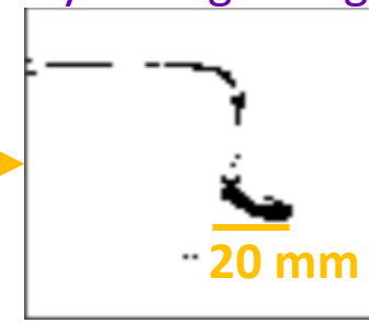
Measure size of defect beyond right edge
