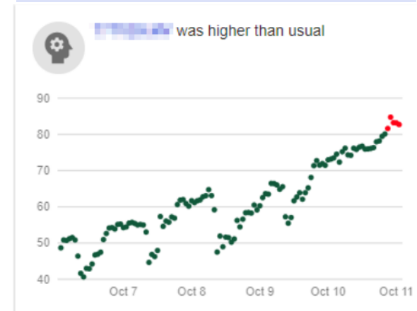
Heater outlet temperature above normal:
