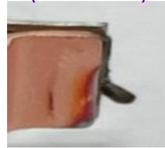
Object with defect (metal burr)
